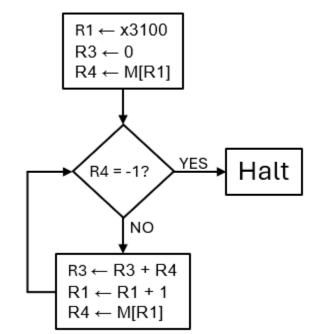
.ORIG x3000 **START** LEA R1, DATA ; R1 < x3100 R3, R3, #0 ; R3 <- 0 AND LDR R4, R1, #0 ; R4 <- M[R1] ; while R4 != -1 LOOP BRn YES (R4 = -1)DONE ; ; do R3, R3, R4 ; R3 <- R3 + R4 ADD ADD R1, R1, #1 ; R1 <- R1 + 1 LDR R4, R1, #0 ; R4 <- M[R1] LOOP BR DONE HALT . END ; Data .ORIG x3100 DATA .FILL **n1** .FILL **n2** ... ... ... . END
